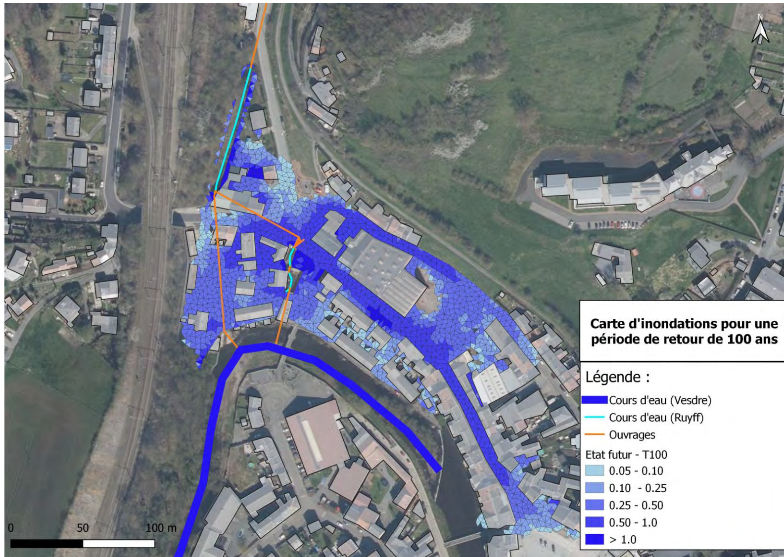
Figure 5.11 - Flood map of the future situation at the most critical time of the flood for a return period of 100 years
