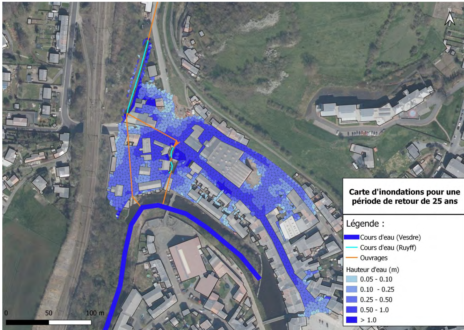
Figure 4.8 - Flood map of the existing situation at the most critical time of the flood for a return period of 25 years.
