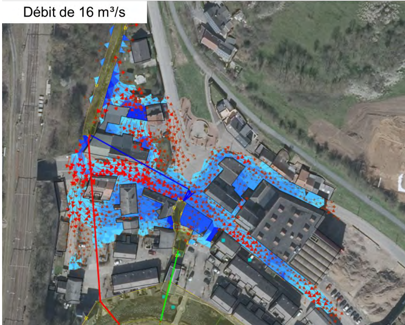
Figure 4.5 -: Propagation of the water in the Vieux-Moulin district once the water has entered the major bed (flow rate of 16 m 3 /s).
