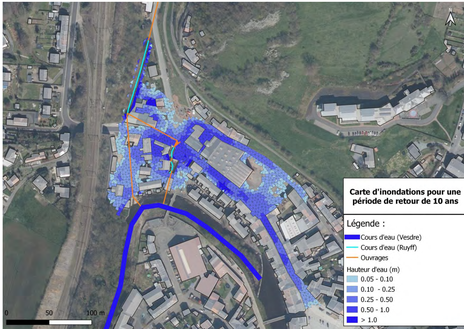
Figure 4.7 - Flood map of the existing situation at the most critical time of the flood for a return period of 10 years.
