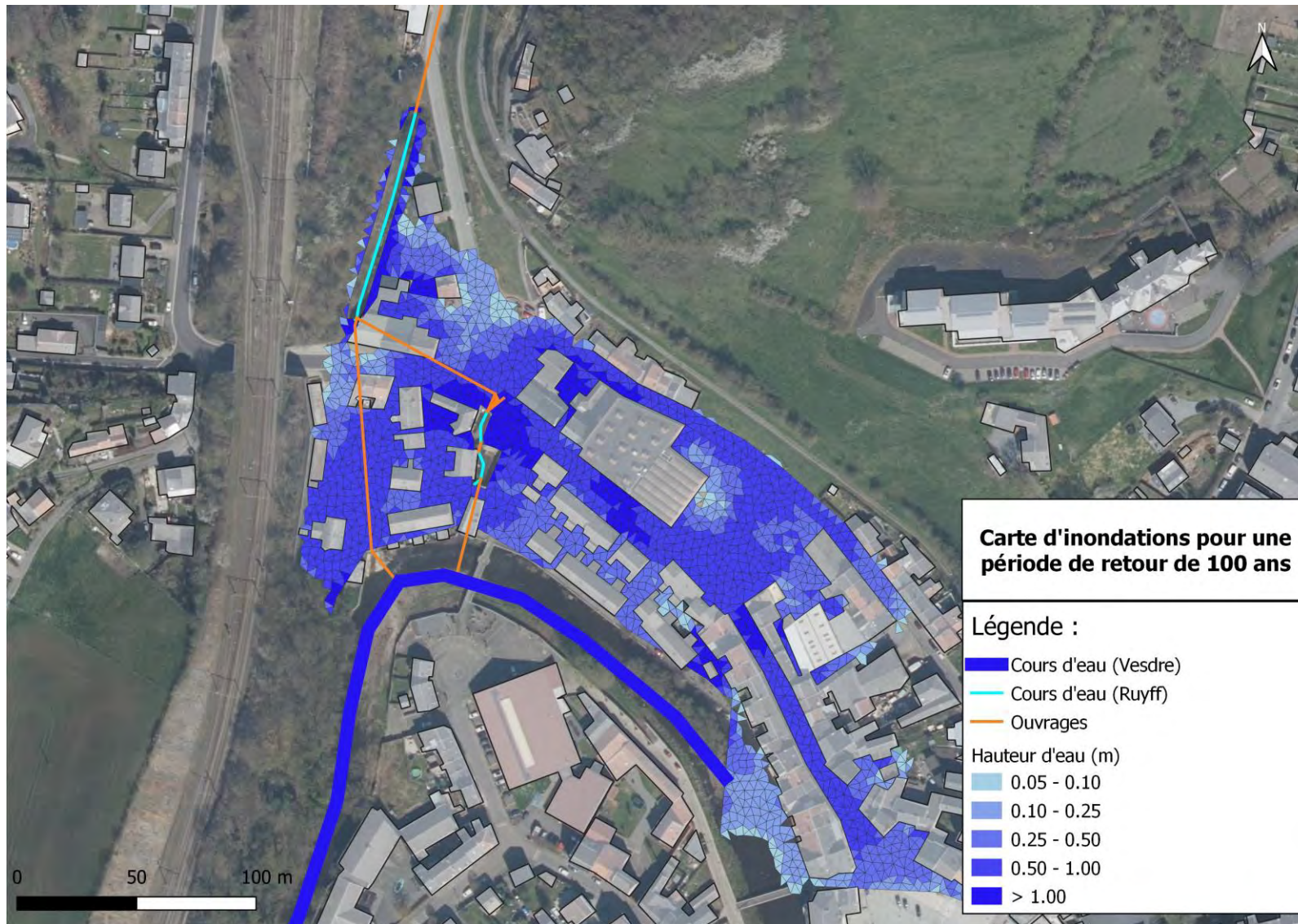
Figure 4.9 - Flood map of the existing situation at the most critical time of the flood for a return period of 100 years.
