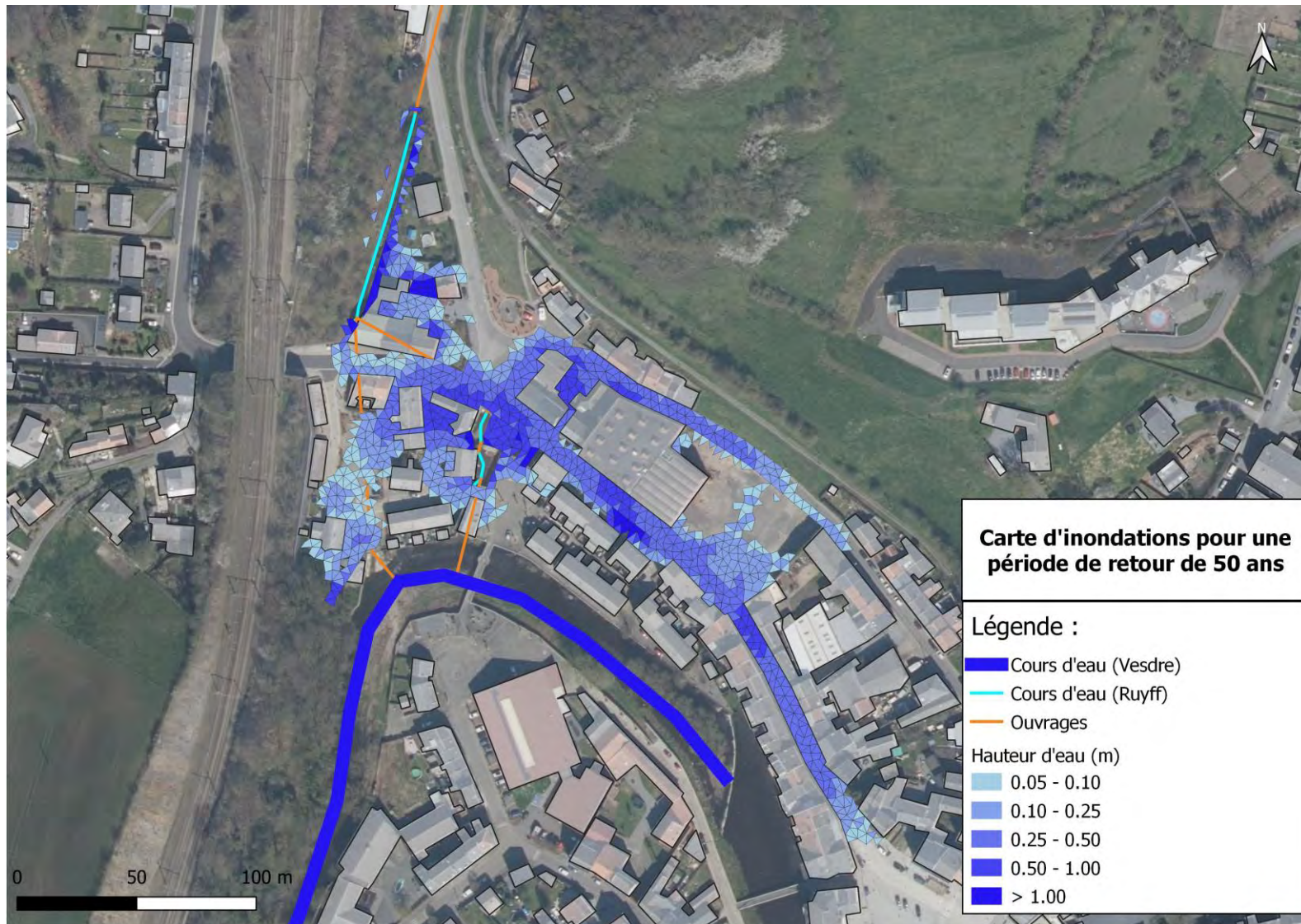
Figure 5.10 - Flood map of the future situation at the most critical time of the flood for a return period of 50 years.
