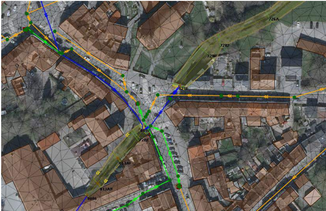
Figure 4-4- Illustration of the integration of the buildings in Soumagne into the major riverbed.
