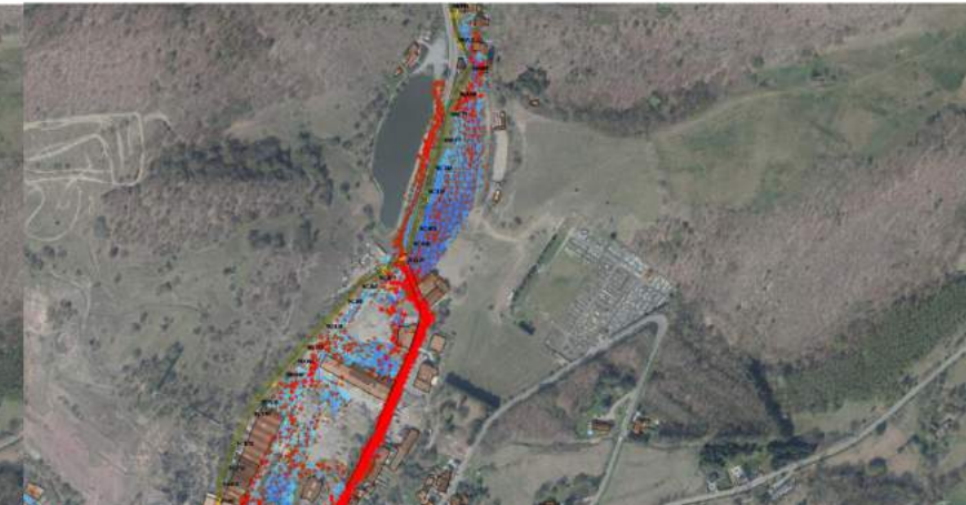
Figure 5-32 : Sequence showing the dynamics of overflows in Rue Noirivaux and Rue sur les Biez (composite rainfall with a 25-year return period)
