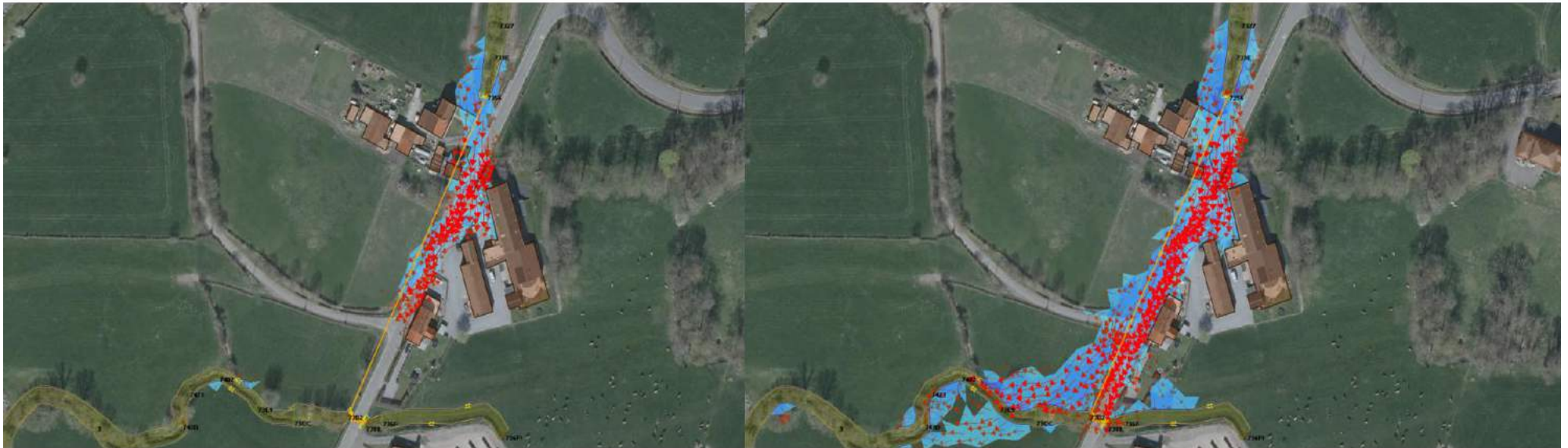
Figure 5-5 : Sequence showing the dynamics of overflows in rue d'Elvaux (5-year return period composite rain)
