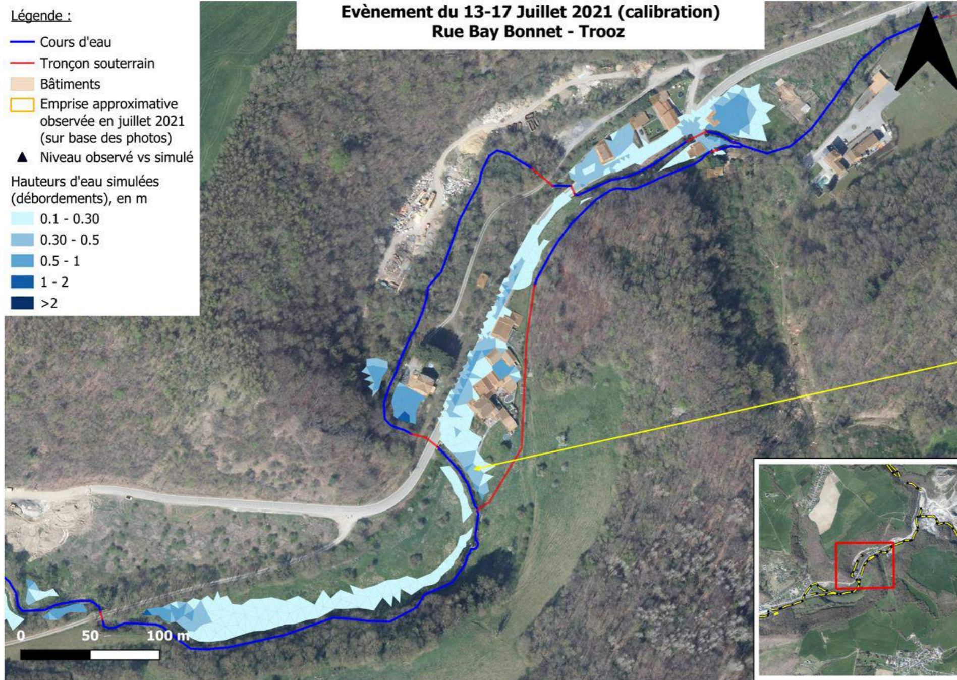
Figure 4-16 : Results of 1D-2D modelling at the most critical moment of the simulation for the July 2021 event at Fond des Gottes in Trooz.
