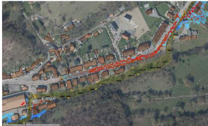
Figure 5-29 : Sequence showing the dynamics of overflows in Rue Fond de Forêt (composite rainfall with a 25-year return period).
