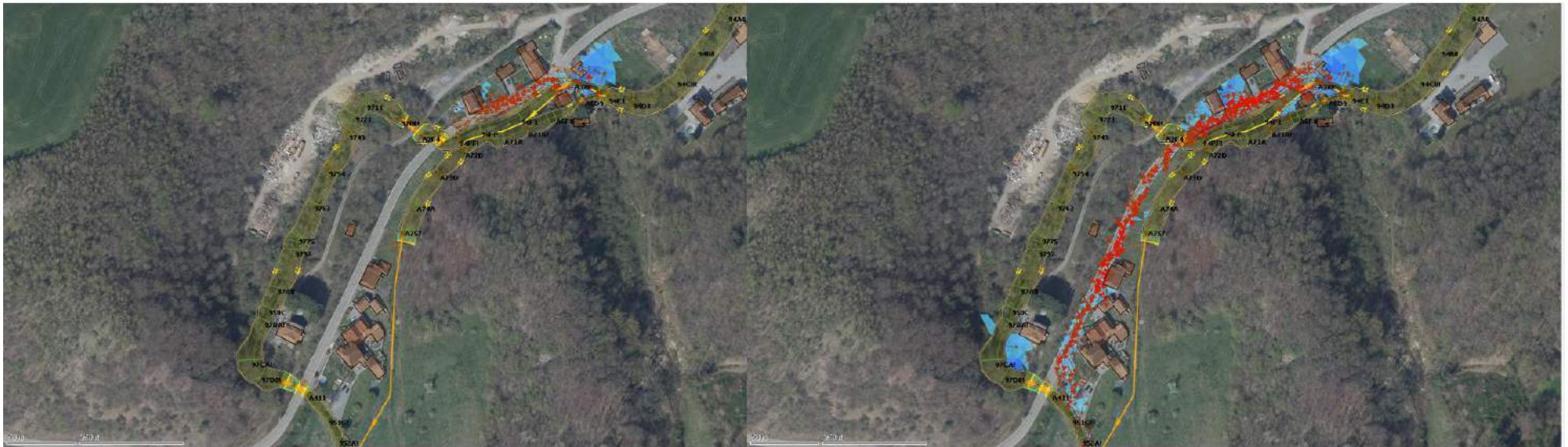
Figure 5-25 : Sequence showing the dynamics of overflows in Rue Bay Bonnet (composite rainfall with a 25-year return period)
