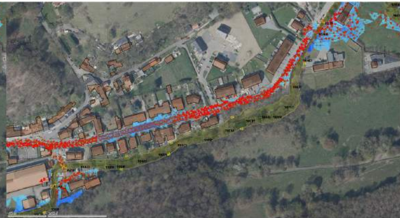
Figure 5-29 : Sequence showing the dynamics of overflows in Rue Fond de Forêt (composite rainfall with a 25-year return period).
