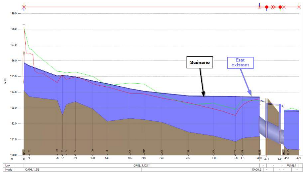
Figure 6-9 : Results of 1D-2D modelling at the most critical time comparing the water line profile of the existing situation (in blue) and the future scenario (in black) for a composite rainfall with a 50-year return period.
