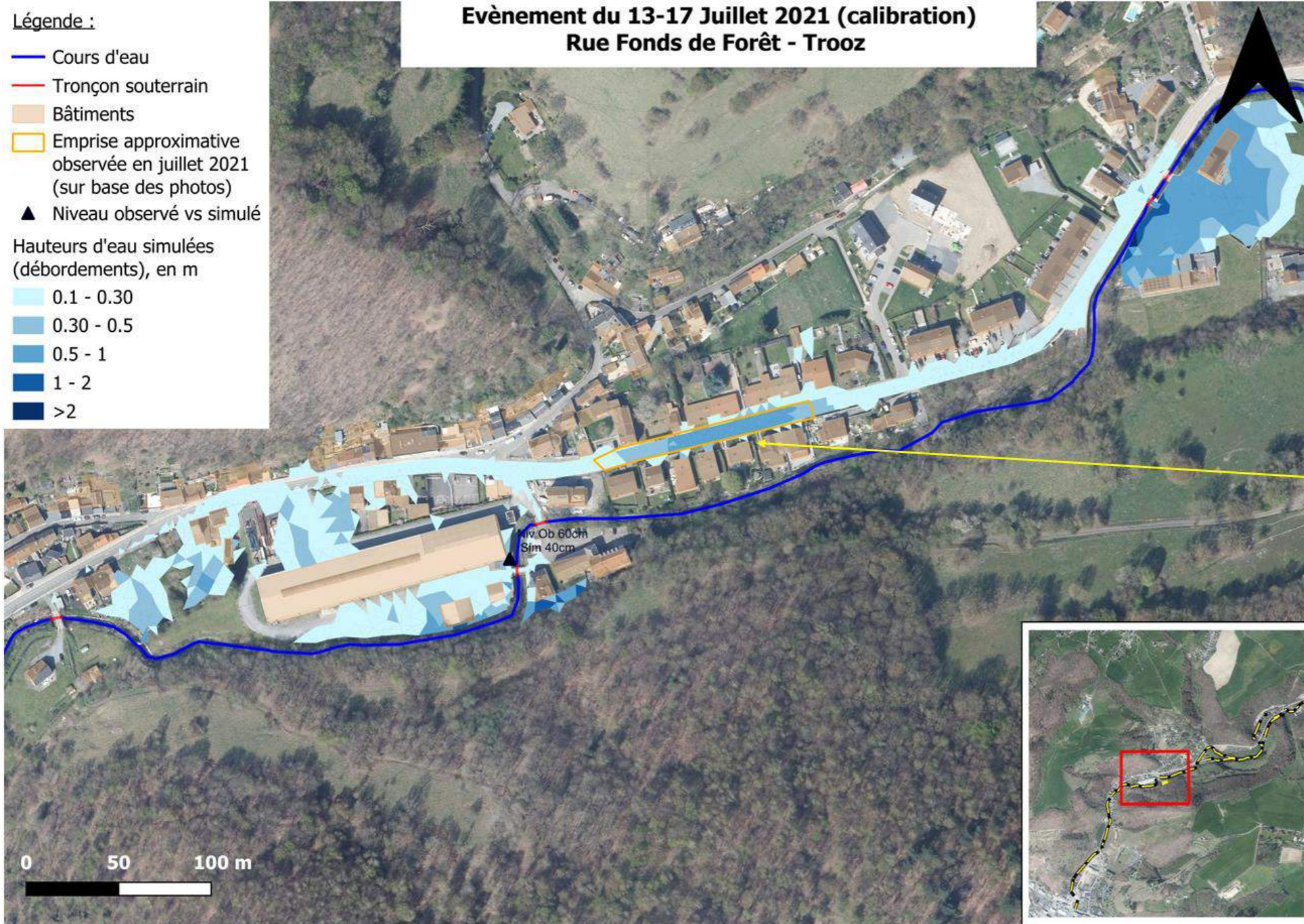
Figure 4-18 : Results of 1D-2D modelling at the most critical moment of the simulation for the July 2021 event at the level of rue Fonds de Forêt in Trooz.
