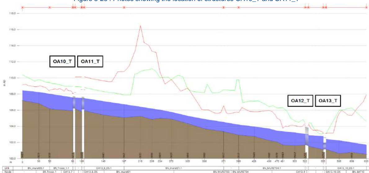
Figure 5-27 : Results of 1D-2D modelling at the most critical point in the simulation, showing the water line profile (in blue) upstream of structures OA10_T, OA11_T, OA12_T and OA13_T (composite rainfall with a 5-year return period).
