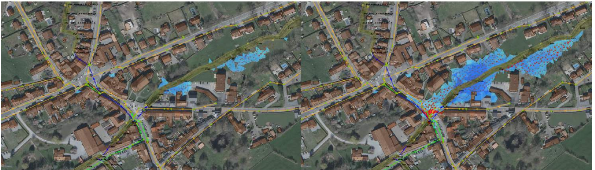
Figure 5-14 : Sequence showing the dynamics of overflows at the level of Place Ferrer in Soumagne (composite rainfall with a 25-year return period).
