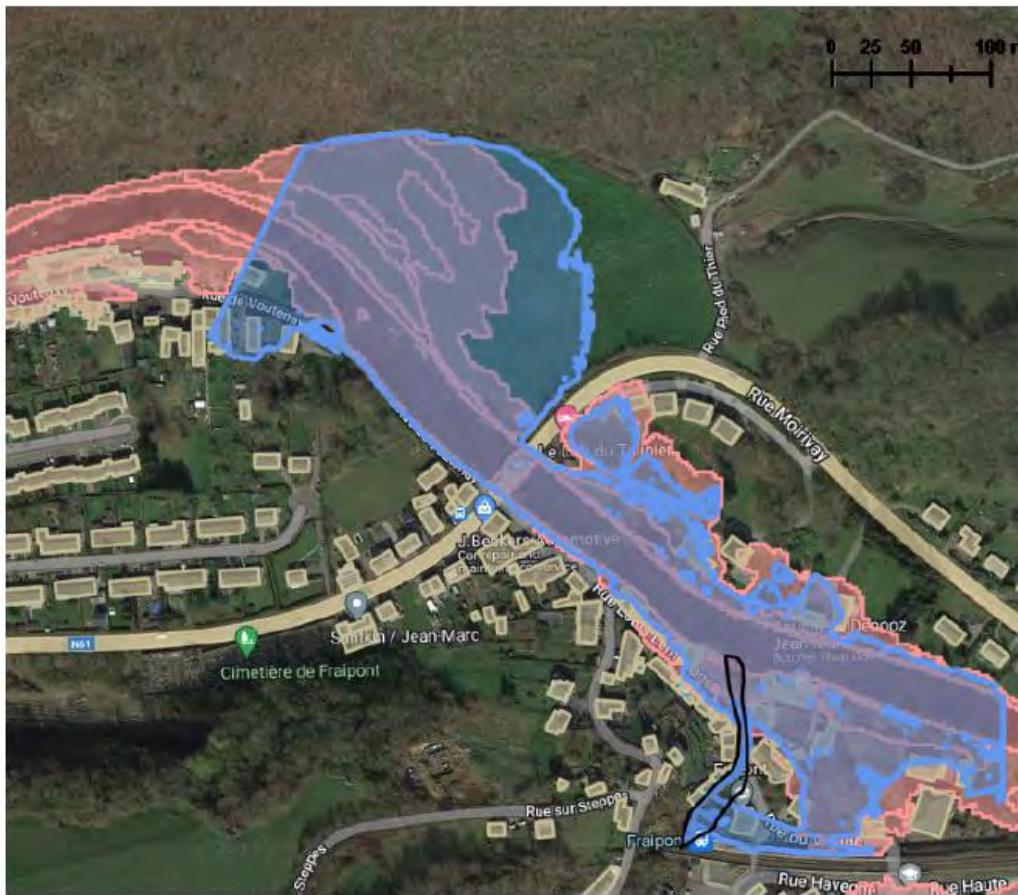
Figure 28 : Comparison between the hazard for the 50-year flood (pink contour, source: https://geoportail.wallonie.be ) and the result of the GEOHECRAS model for the same return period (blue contour).
