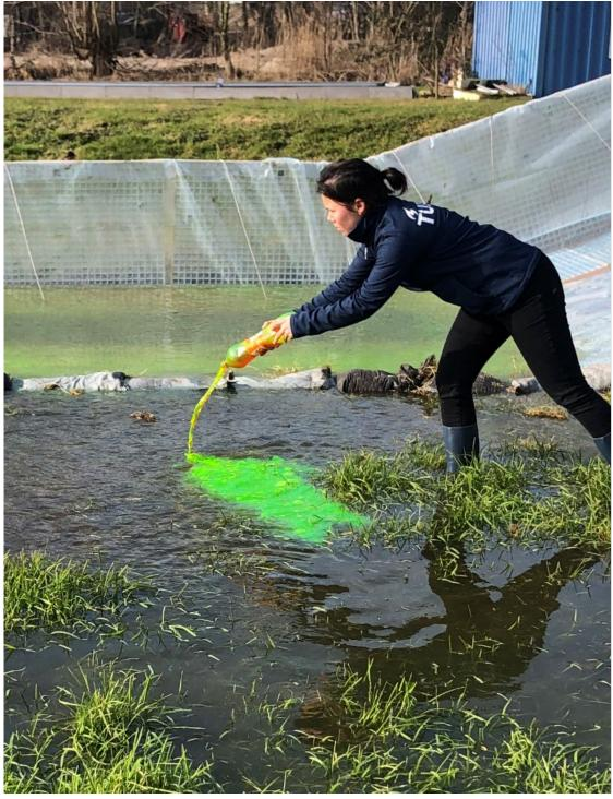
Figure 20 Test with tracer fluid at Flood Proof Holland together with the Waterboard Limburg
