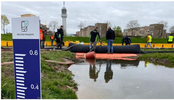
Figure 12: Temporary Flood barrier testing April 6th, 2022, at the Groene Rivier Site in Roermond
