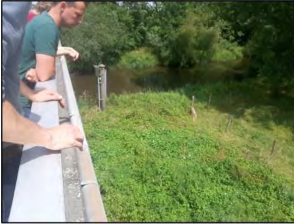
Plate 10. View looking upstream from the bridge carrying the N293 road across the Roer near the village of Sint Odilienberg. The green pole on the riverbank, centre-left, contains the 2.H.2 stage gauge.
