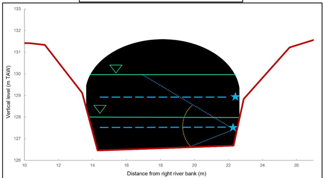
Figure 3.3 Conceptual design of a possible station set-up with two side looking Doppler systems deployed under the road bridge, with (top) a detailed map of the area around the bridge (as in Figure 3.2), (middle) a legend, and (bottom) a cross sectional area. The bed level profile is obtained from profile P417 in Figure 3.2.
