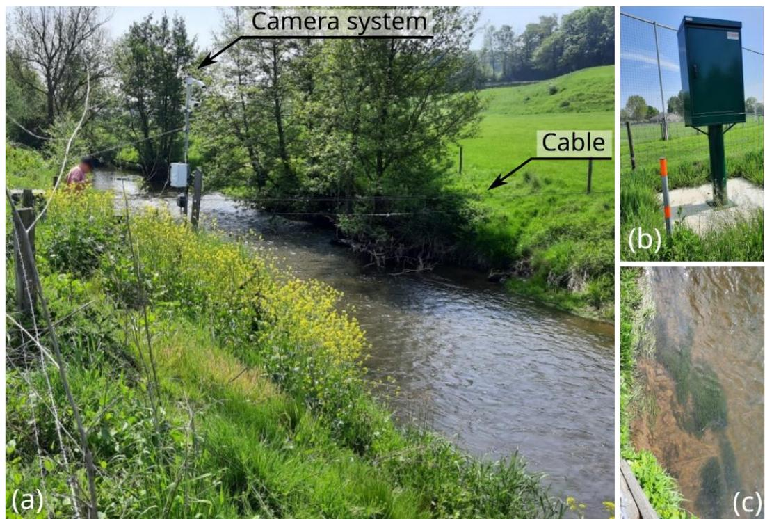
Figure 3.4 (a) Overview of the discharge measurement station in the Geul near Hommerich. Discharge measurements are derived with a rating-curve, and a camera system. In addition, the measurement station is regularly calibrated with moving boat ADCP measurements along a cable. (b) A reliable rating-curve is obtained with the water level sensor. (c) The bottom is relatively stable in the Geul near Hommerich. However, there is still growth of vegetation on the bottom of the Geul.
