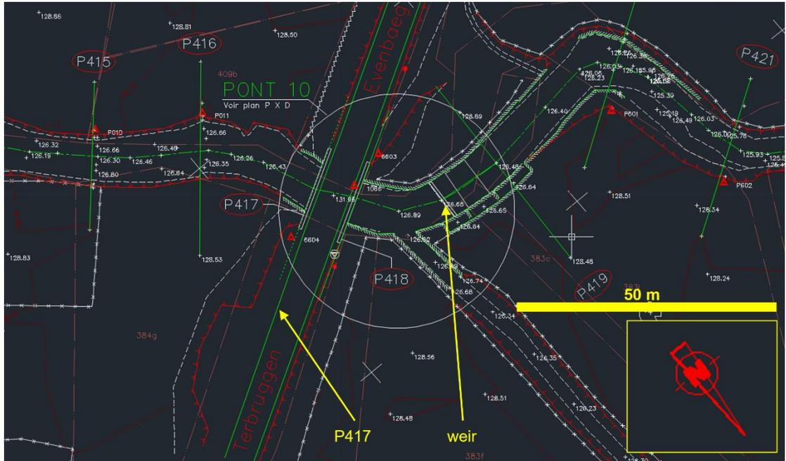
Figure 3.2 Map of the Geul at Sippenaeken, flow being from left to right. The road bridge is situated upstream of the weir. A channel branches off the Geul in between the bridge and the weir, which is usually closed with gates. (Source: Ministère de la région Wallonie, SPW, 1/500 map, dated: March 1994).
