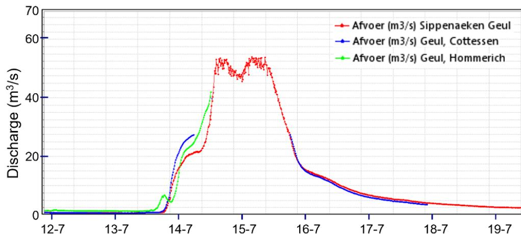
Figure 1.1 The monitored discharges at three locations along the Geul during the high discharge event in 2021. (source: (van Heeringen et al., 2022)).
