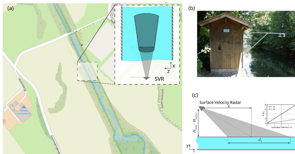
Figure 3.5 (a) Conceptual design for Hommerich. (b) A sensor mounted on a cantilever beam (adapted from: OTT HydroMet (2006)). (c) The SVR spot size depends on the height above the fluid level.
