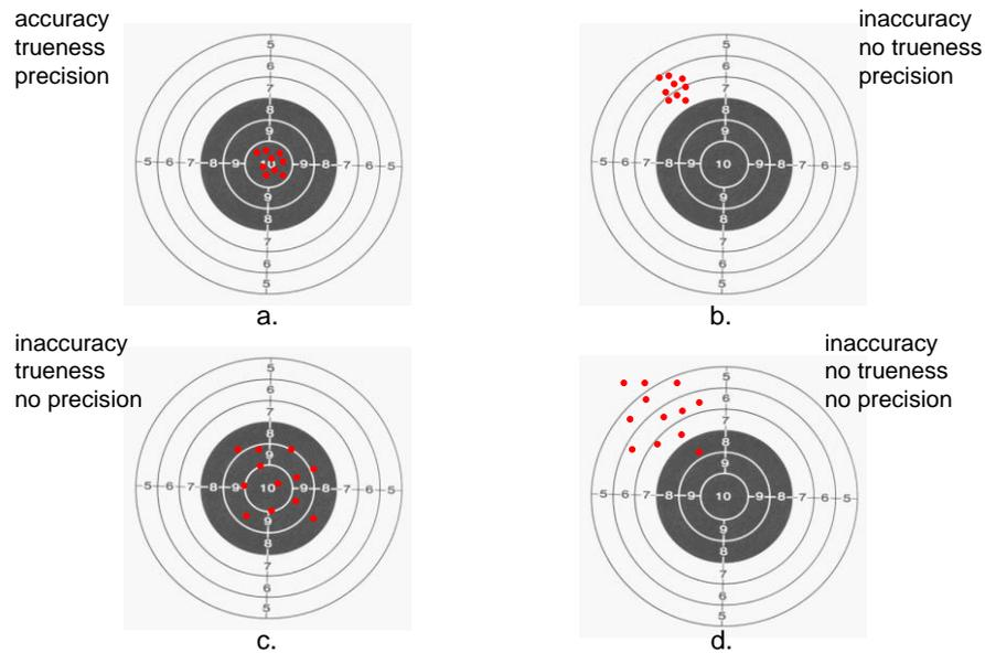
Figure 1.6 Characterization of accuracy, trueness, and precision in a set of measurements (source: (Bertrand-Krajewski et al., 2021)).
