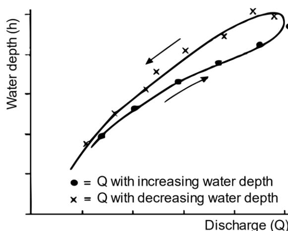
Figure 2.1 Hysteresis of the rating-curve during extreme conditions (adapted from Boiten et al., 1995).
