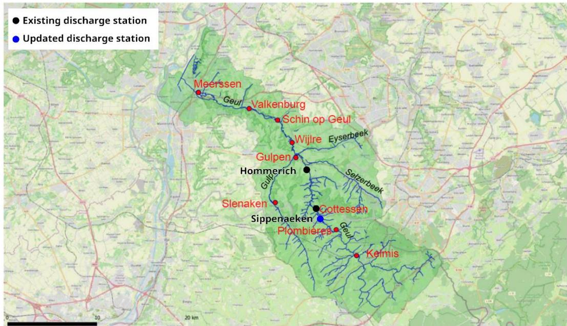
Figure 1.2 The catchment area of the Geul, with the discharge measurement stations indicated. (adapted from: Asselman & Van Heeringen (2023)).
