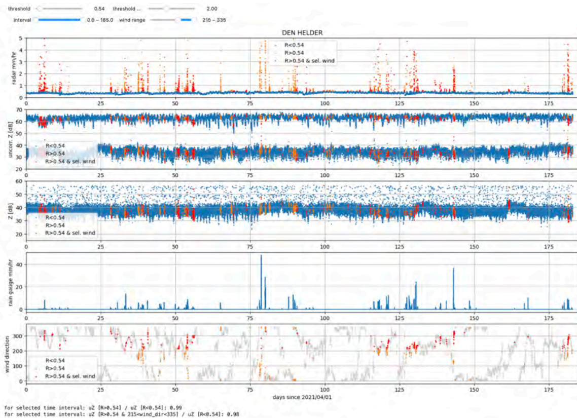
Figure 3.5: Radar-derived rainfall intensity at the radome (row 1), uncorrected (row 2) and corrected (row 3) radar reflectivity factors, rain gauge rainfall intensity (row 4), and wind direction (row 5) for the Den Helder radar for 185 consecutive days in 2021.
