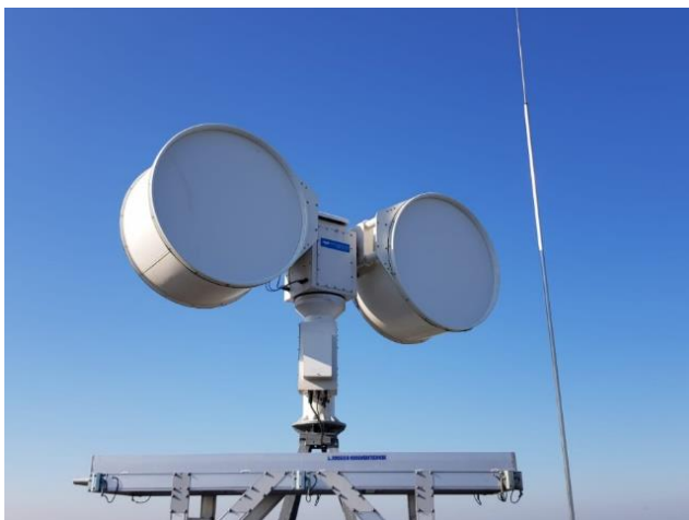
Figure 2- X-band rain radar (Rijnmond) located in Rotterdam
